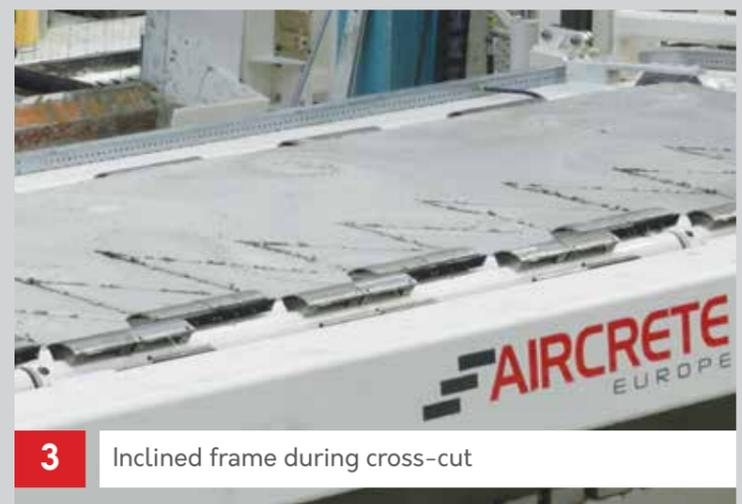
3 Inclined frame during cross-cut
