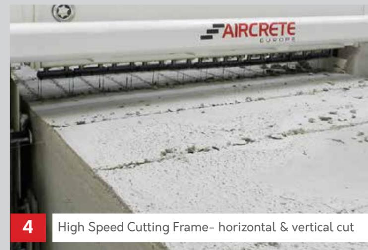
4 High Speed Cutting Frame- horizontal & vertical cut
